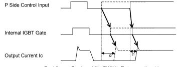
Real line…off pulse width>PWIN(off); turn on time t1 Broken line…off pulse width<PWIN(off); turn on time t2 Fig. 5 Timing Charts of The DIPIPM Protective Functions
