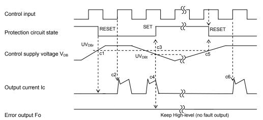
[D] UV protection sequence for Brake circuit (UV<sub>D</sub>)
