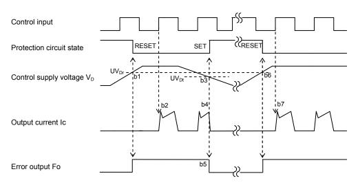
[C] Under-Voltage Protection (P-side, UV<sub>DB</sub>)
