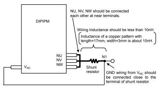
Low inductance shunt resistor like surface mounted (SMD) type is recommended.
