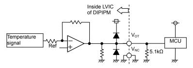
V<sub>OT</sub> outputs the analog signal that is amplified signal of temperature detecting element on LVIC by inverting amplifier.
