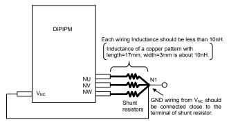
Low inductance shunt resistor like surface mounted (SMD) type is recommended. Protection current level  $I_{SC}$  changes by inserting shunt resistor.
